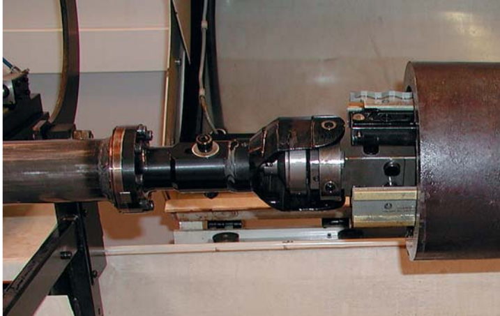
9 Large workpieces in fixed position being honed with double universal joint.
