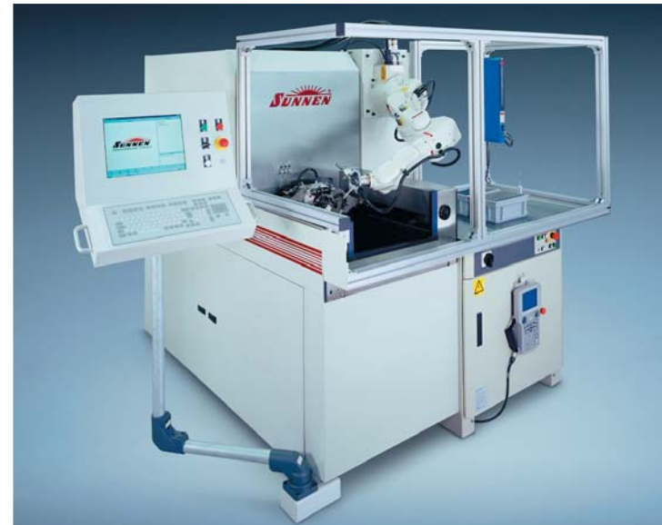
◀ 28 More and more, six-axis knee-action robots are being used for flexible automation of honing machines.
