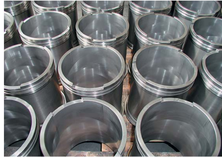
12 Thin-walled cylinder sleeves are honed with low cutting pressure and minimal heat development to microinch accuracy.
