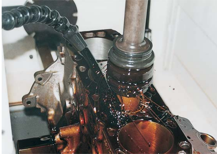
5 ► Honing removal stock with low pressure and large flow of cutting oil.
