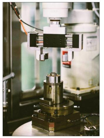
After each bore is honed and airgaged as acceptable, a robot inside the honing machine's work envelope rotates the workpiece to align the next bore for the honing tool operator would hone one bore, clean the part, air gage it at three different levels and then at 90 degrees bottom/middle/top
