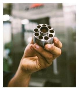
The heart of a hydraulic piston pump, called a cylinder block or rotor, starts as a turned blank up to eight inches diameter. Then, nine circumferential piston bores from 0.1875" to 1.5" (4.8 - 38.1 mm) diameter are roughed in on a machining center, and the part may be heat treated.
