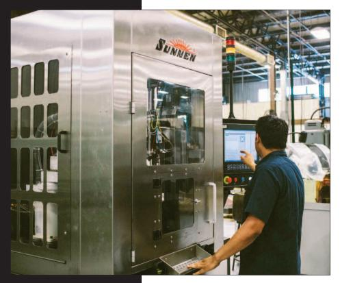
Sunnen's new multi-feed control technology allows the user to select the better tool feed option – rate feeding or force feeding – to suit the workpiece geometry, material and tool type/size.
